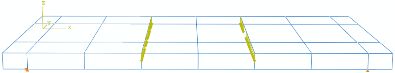
Figure 9 - Intermediate floor load test: green arrows: load, orange points: restraints
