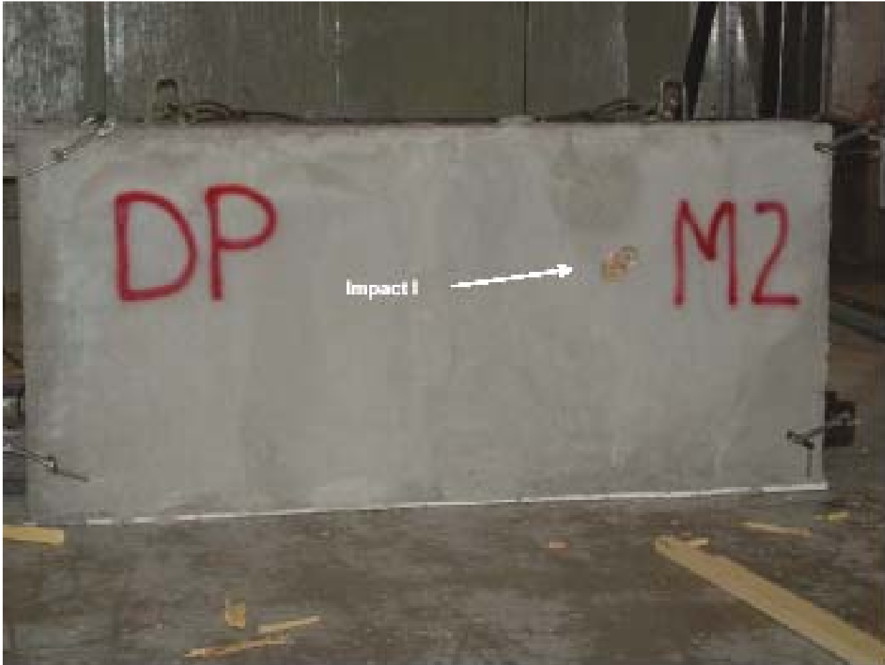
Series 3 Panel Impacted by Tornado Missile I
