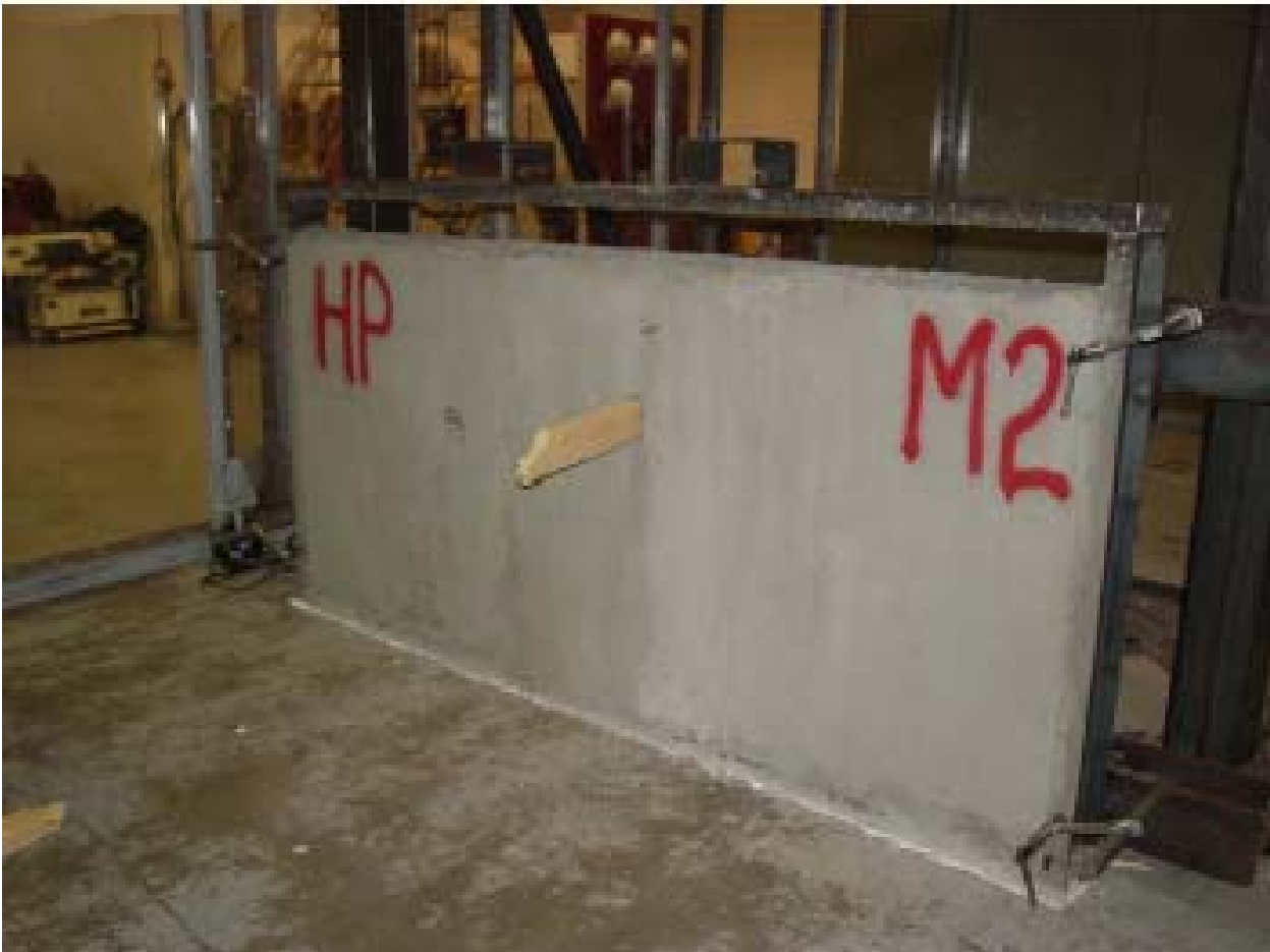
Series 2 Panel Impacted by the Second Hurricane Shelter Missile
