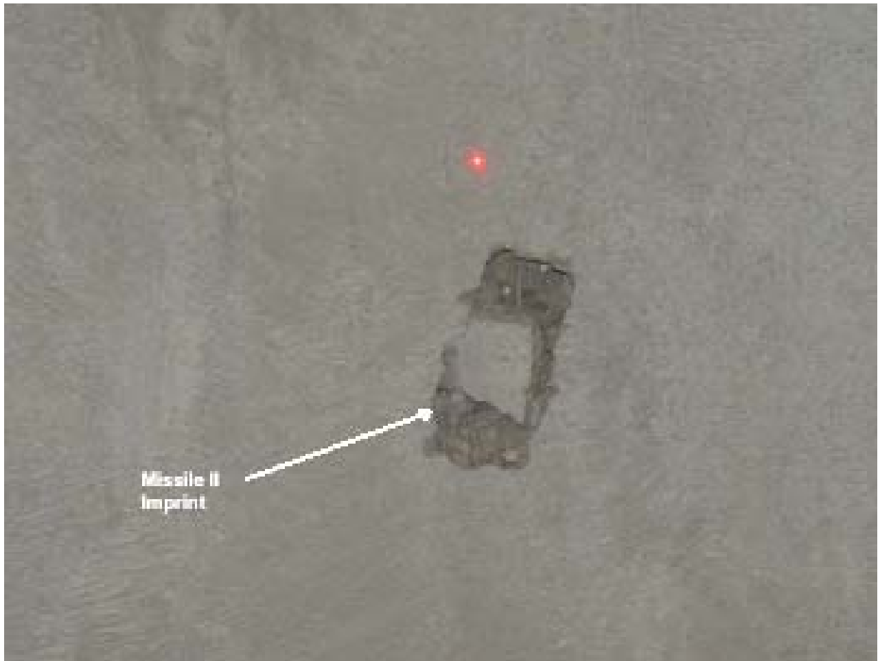
Impact Face of Series 1 Panel after Missile II
