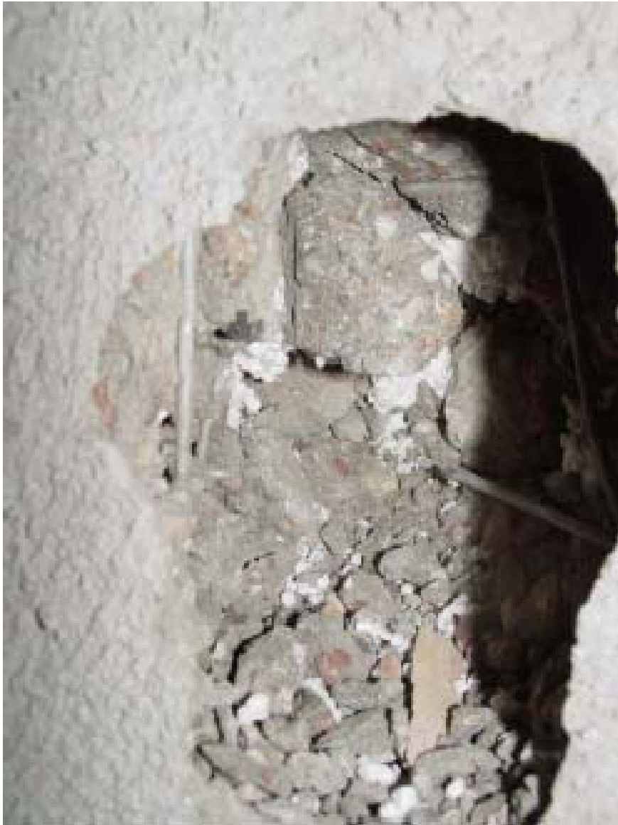
Impact Hole from Series 2 Hurricane Shelter Missile
