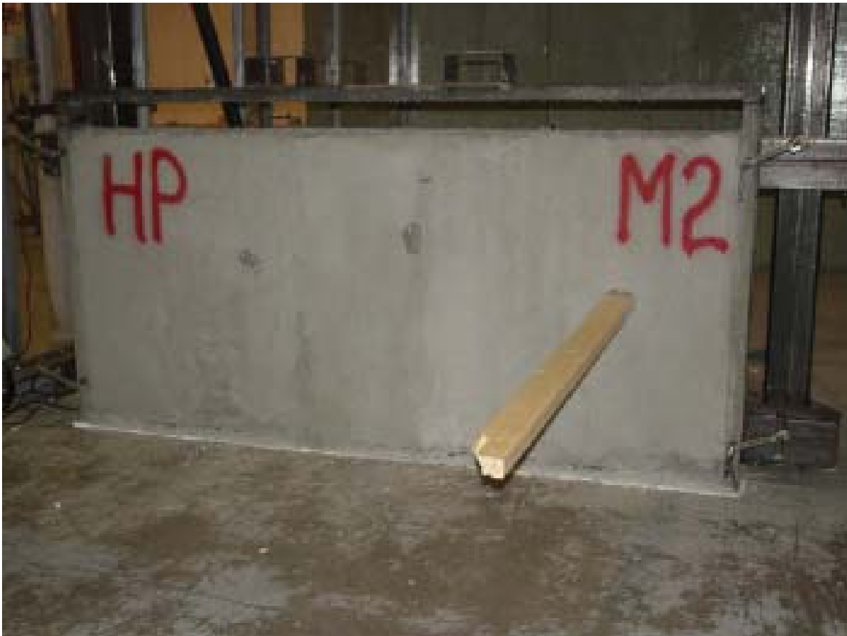
Series 2 Protocol 2 Hurricane Shelter Impact III
