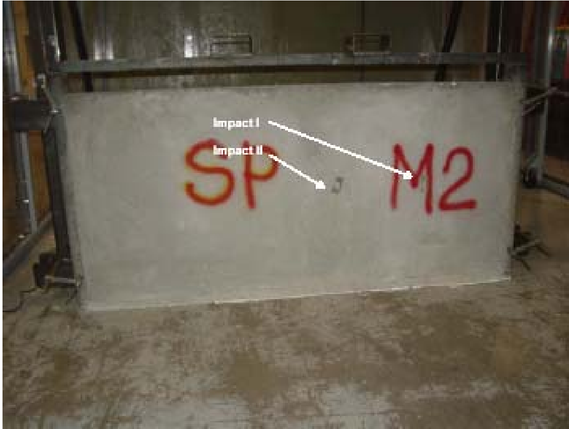
Series 1 Specimen Impacted by Hurricane Protocol Missile II
