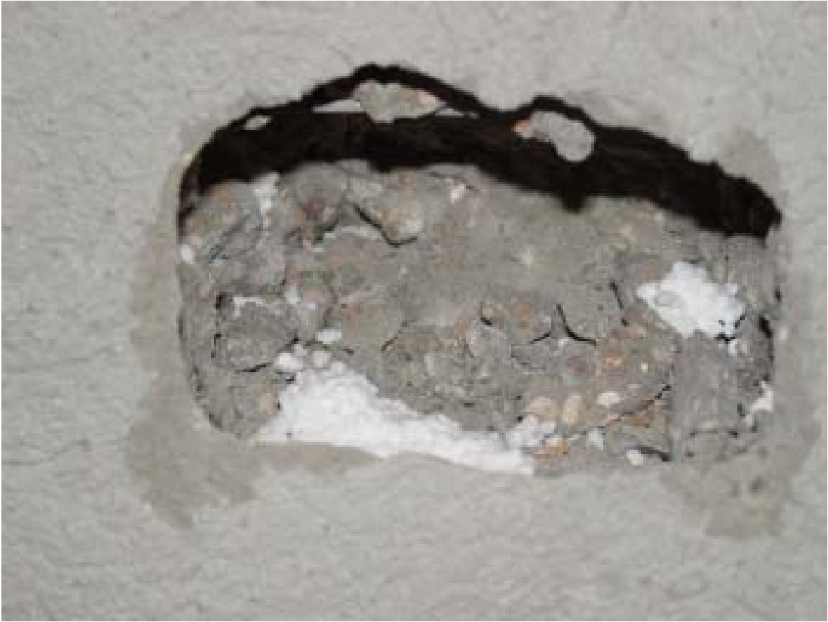
Impact Damage from Missile III on Series 2 Protocol 2
