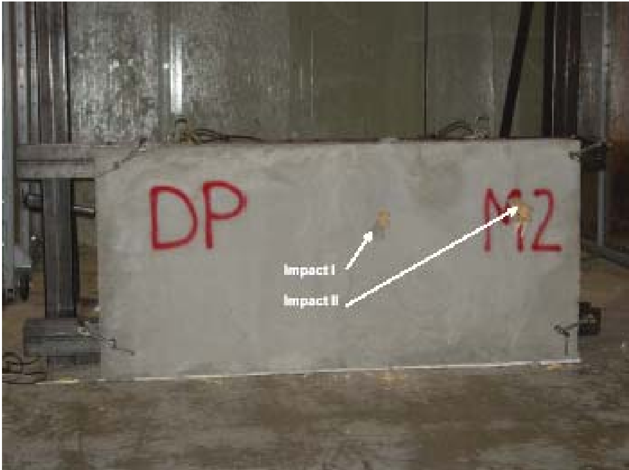
Series 3 Panel Impacted by the Second Tornado Missile
