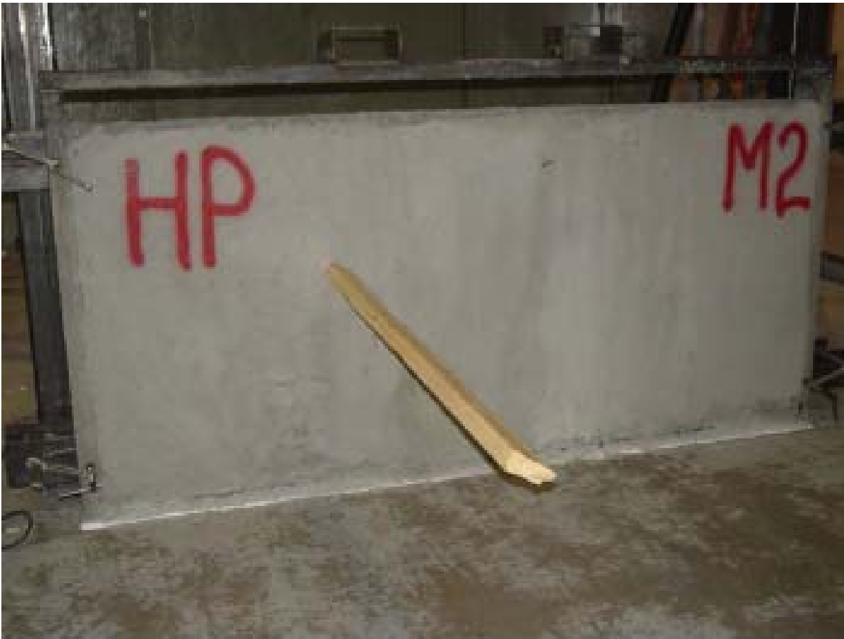
Hurricane Shelter Impact on Series 2 Specimen
