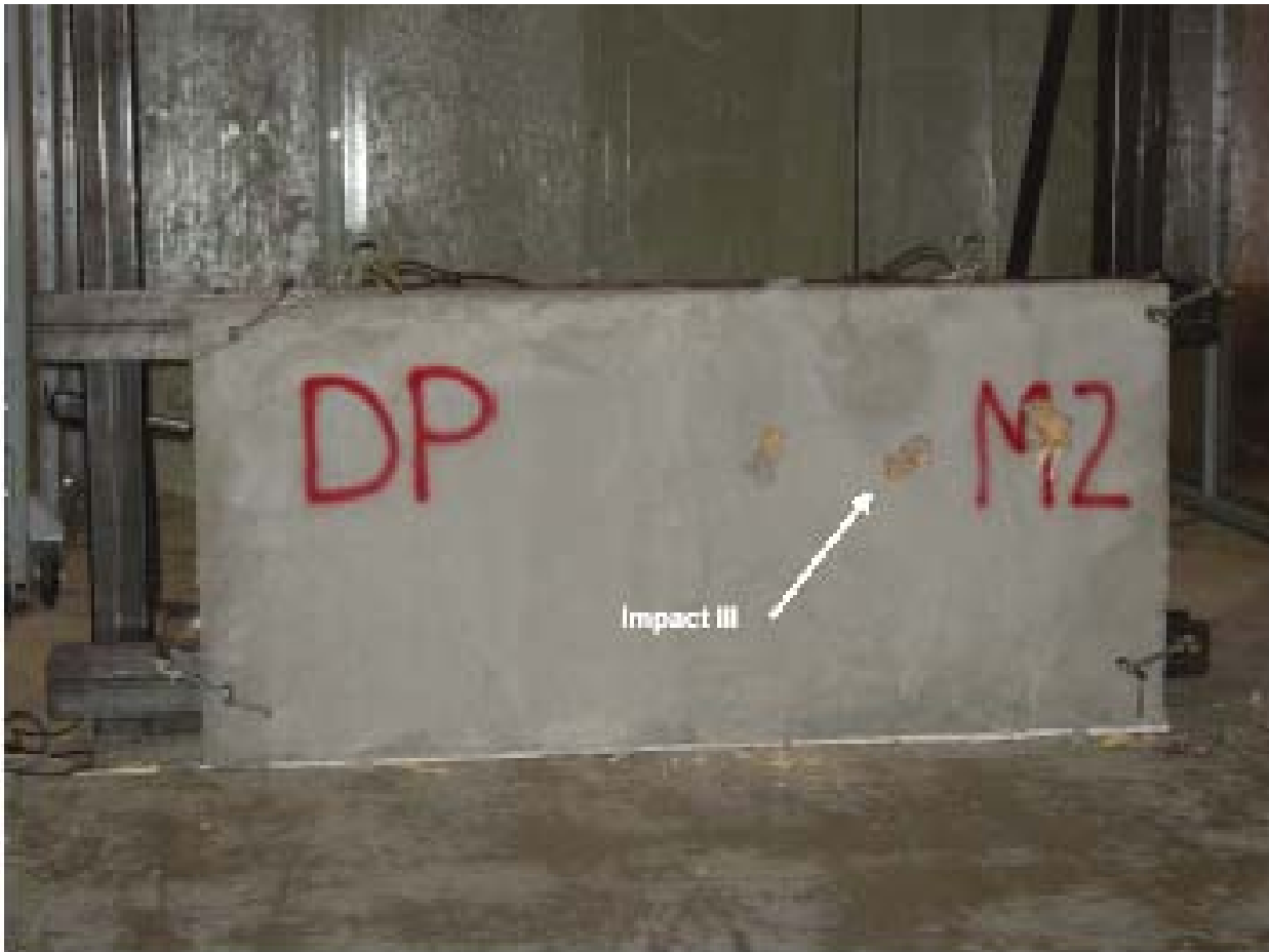
Series 3 Panel Impacted by the Third Tornado Missile
