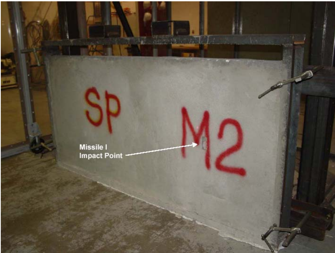
Series 1 Panel Impacted by Missile I
