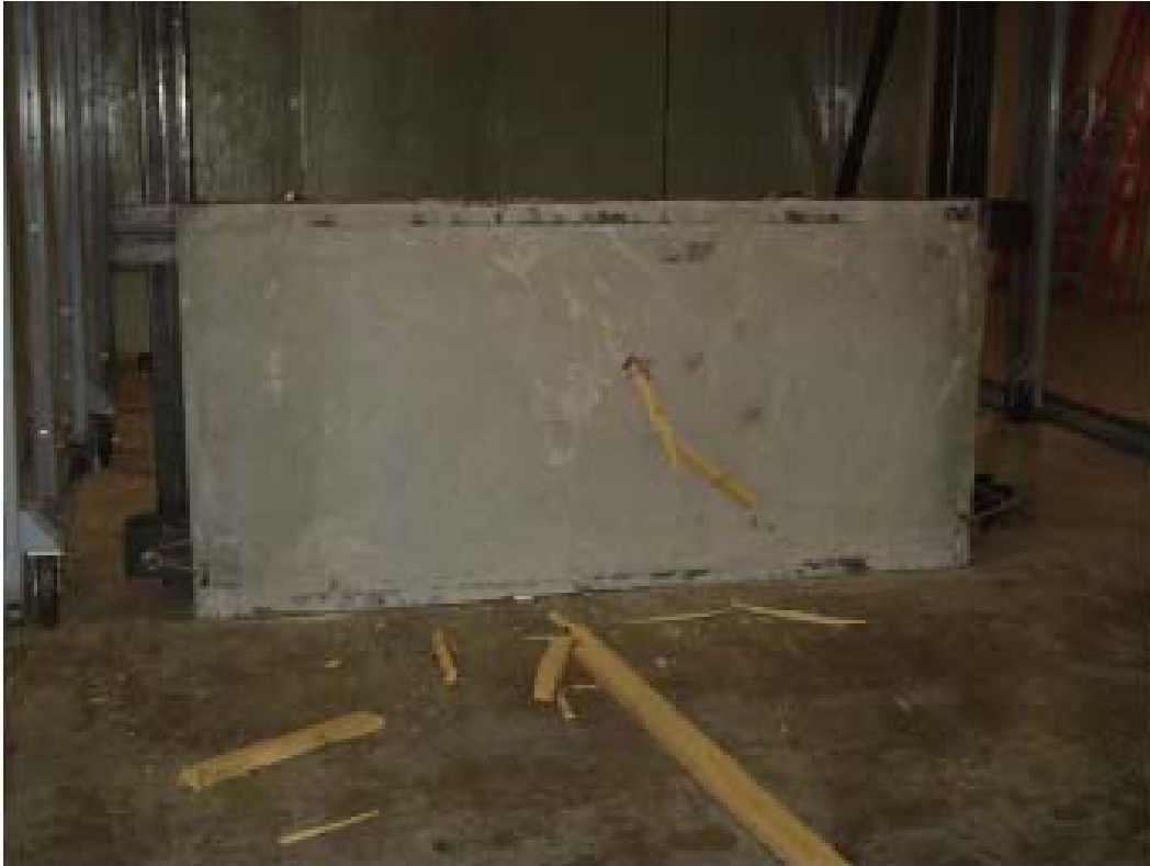
Series 5 Protocol 1 Tornado Missile I Impact on Panel
