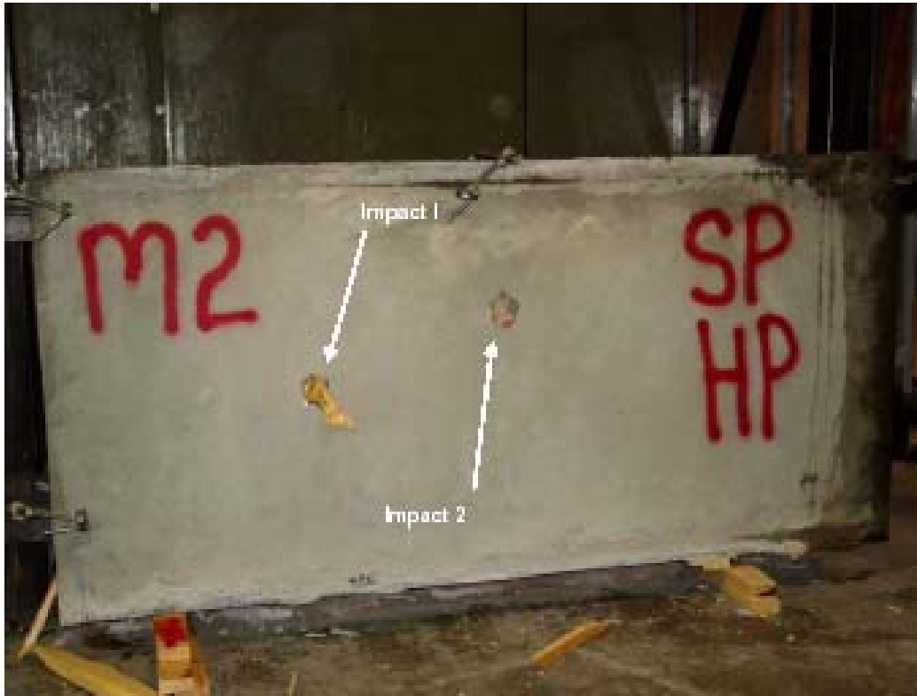
Series 2 Impact by Tornado Shelter Missile II
