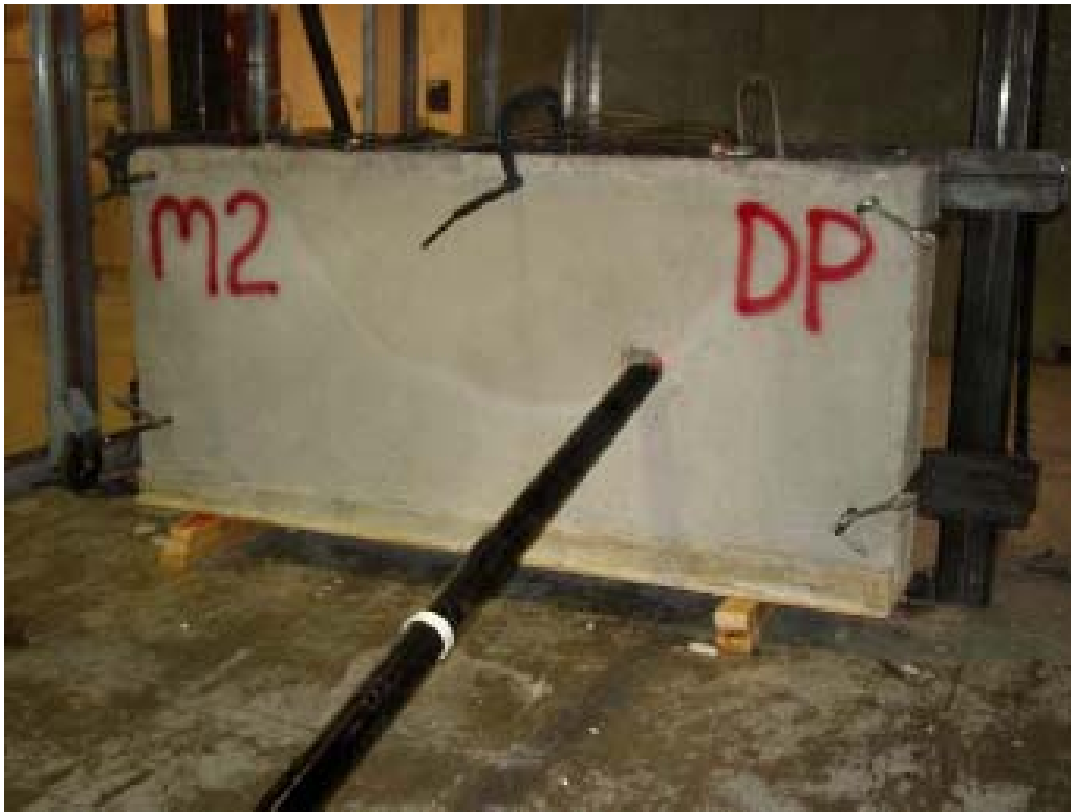
Series 3 Panel Impacted by the Nuclear Regulatory Missile
