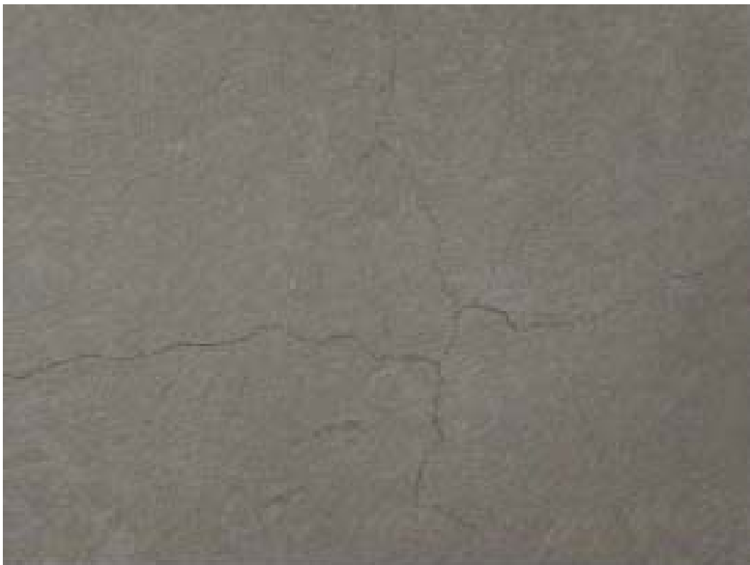
Radial Cracking on Backside of Series 3 Impact Specimen
