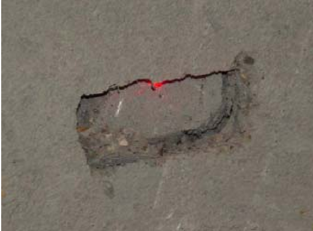
Series 5 Panel Impacted by the Tornado Missile II
