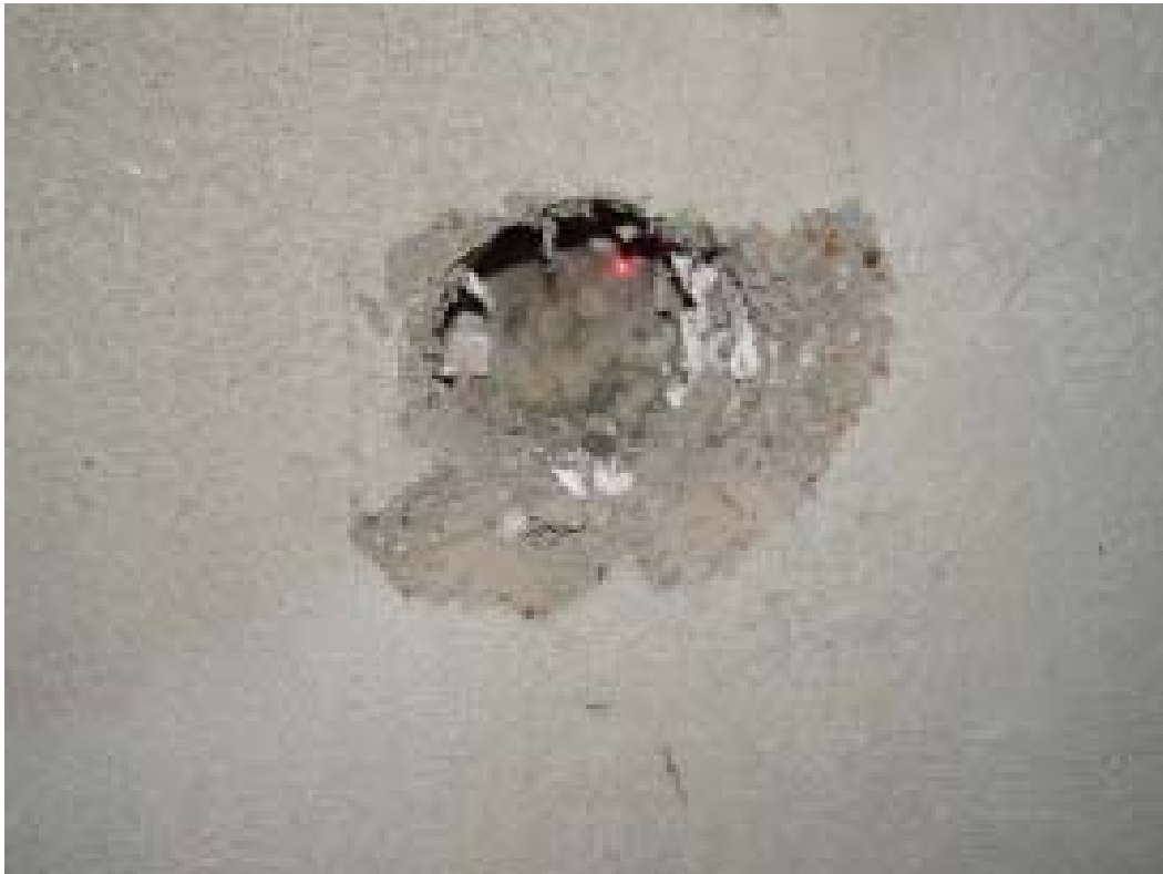
Impact Crater from Series 2 Nuclear Regulatory Missile
