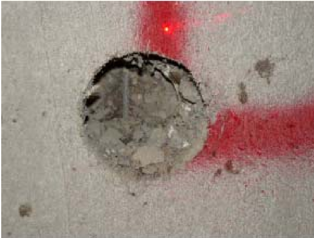
Impact Damage from Missile I on Series 4 Protocol 5a
