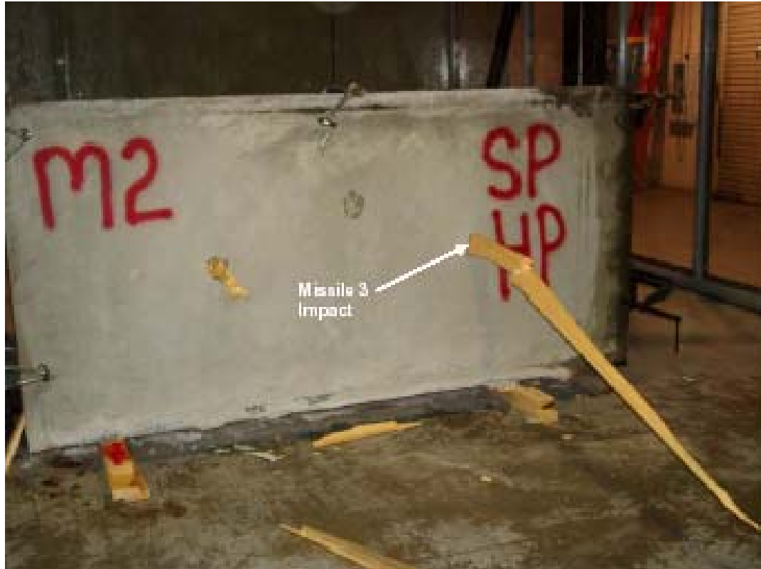
Tornado Shelter Impact on Series 2 Specimen
