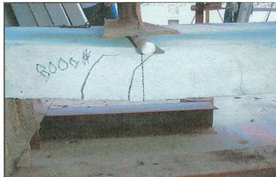
Illustration 3.11 – Crack at one quarter of panel length during the bending test
