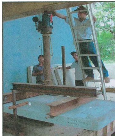
Illustration 3.10 – Installation of the load system for bending test
