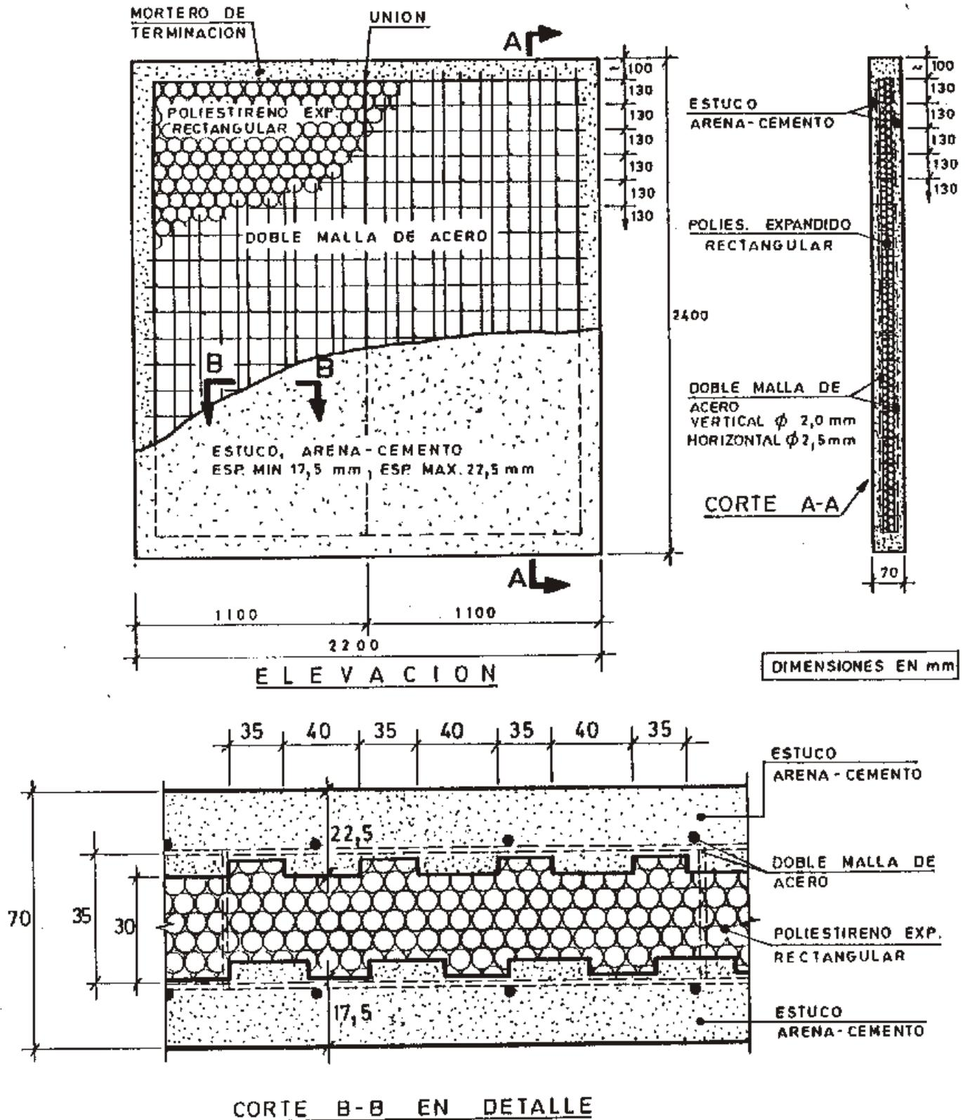
FIG. 1. ELEVACION, CORTE Y DETALLE DEL ELEMENTO.
